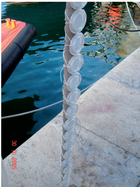
Figure 2. Arrangement of Chemcatcher samplers for deployment.
